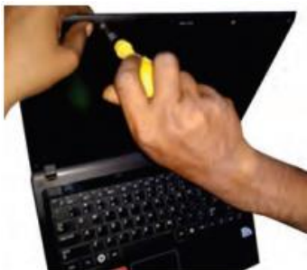
Fig. 3.78: Remove the four screws securing LCD screen
