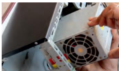
Fig. 3.4: Insert power supply
