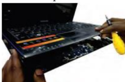
Fig. 3.61: Separate palm rest from bottom case
