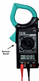
Fig. 4.17 Setting the rotary selector on the clamp meter
