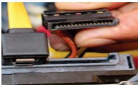
Fig. 3.49: Unplug power cable from optical drive and HDD
