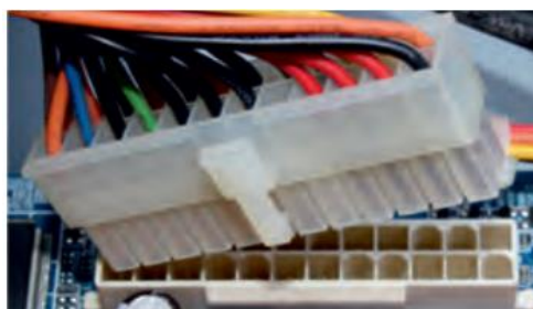
Fig. 3.18: Plug-in 20-pin ATX power connector to motherboard
