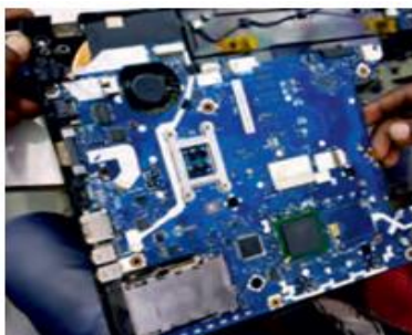
Fig. 3.75: Remove the motherboard from notebook case
