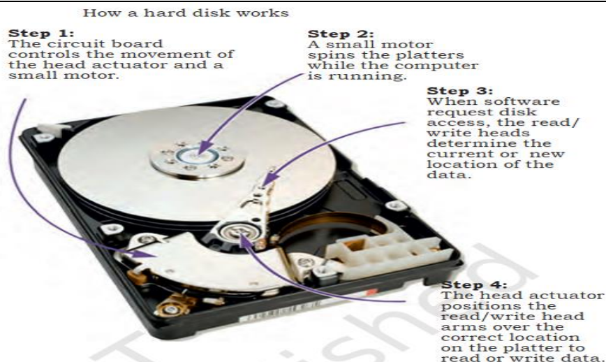
Fig. 4.11: working of hard disk
