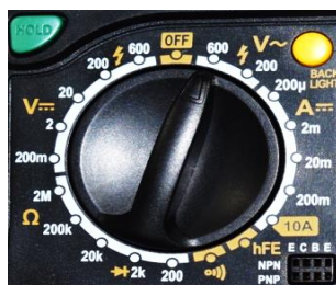
Fig. 4.26 (b) Turning the knob to measure the AC voltage
