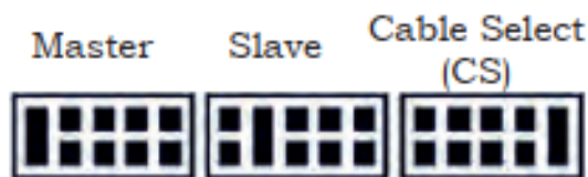
Fig. 4.32: Master and slave cable select
