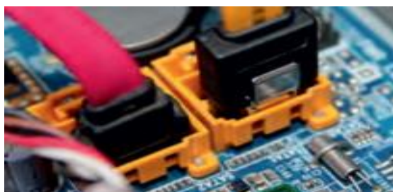
Fig. 3.48: Unplug SATA cables from motherboard
