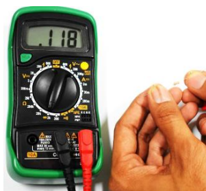
Fig. 4.23 Measuring the resistance of resistor by touching the resistor terminal to the red and black probes
