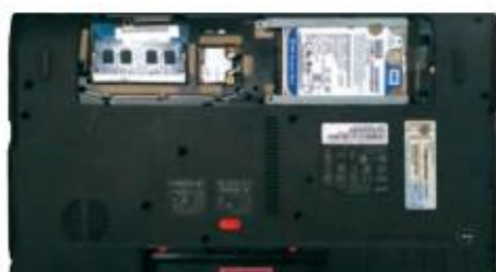
Fig. 3.62: Remove screw from the hard drive and disconnect it
