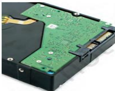
Fig. 4.34: Back of SATA HDD
