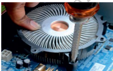
Fig. 2.34.: Screwing the heat sink
