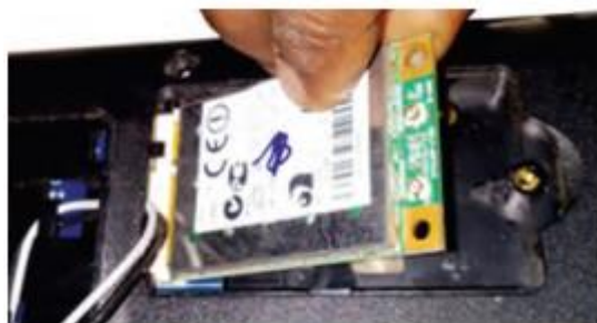
Fig. 3.73: Disconnect Wi-Fi Module
