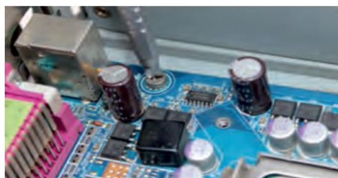
Fig. 3.11: Tighten all the motherboards screws
