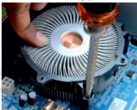
Fig. 3.7: Screw the heat sink
