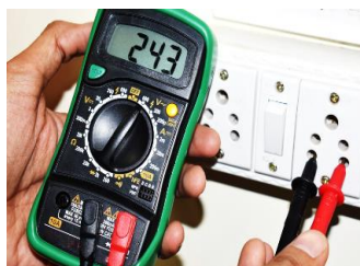
Fig. 4.27 Measuring AC voltage using multimeter
