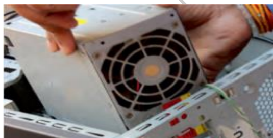
Fig. 3.51: Unscrew the SMPS and remove it from cabinet
