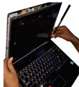
Fig. 3.78: Remove the four screws securing LCD screen
