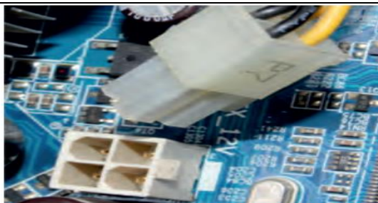
Fig. 3.19: Plug-in 4-pin AUX power connector to motherboard
