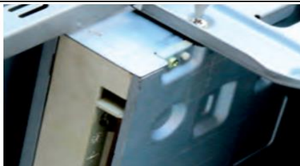
Fig. 3.15: Tighten screws of optical drive
