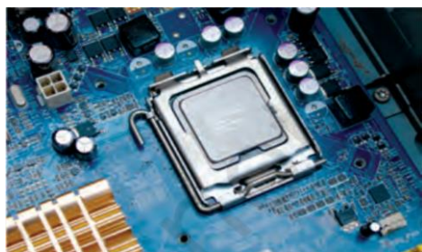
Fig.2.31: Installing CPU on the motherboard
