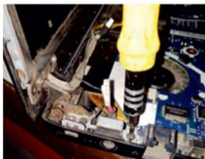
Fig. 3.71: Open the hinge and remove DC power jack
