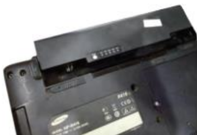
Fig. 3.60: Remove battery and optical drive
