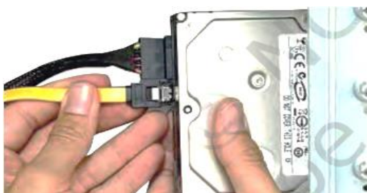
Fig. 4.17 Connecting SATA-data cable
