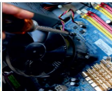
Fig. 3.8 Screw the heat sink fan assembly
