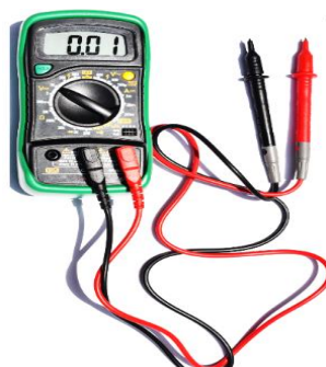
Fig. 4.35 Connecting the red probe to the volt terminal and black probe to the common terminal
