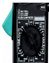
Fig. 4.18 Setting the clamp meter to voltage
