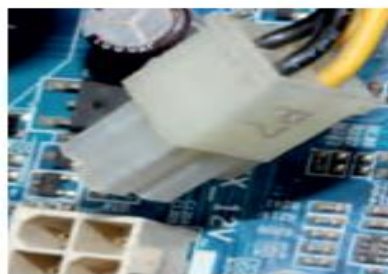
Fig. 3.47: unplug 4-pins AUX power
