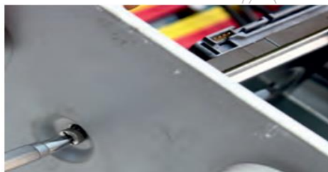
Fig. 3.13: Tighten screw of HDD
