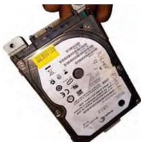
Fig. 3.64: Remove hard drive assembly
