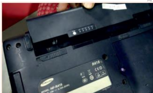
Fig. 4.19: Remove battery and optical drive
