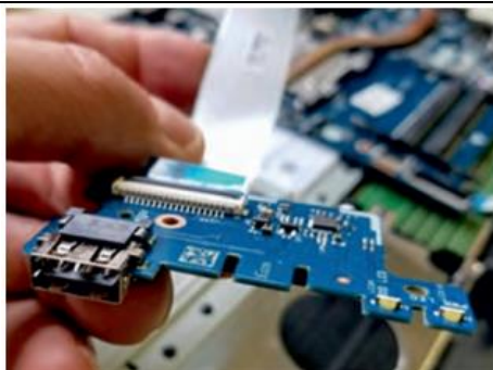
Fig. 3.67: Remove USB LED status board
