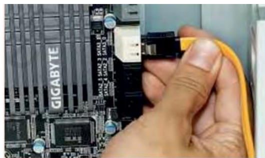
Fig. 4.18: Plugging SATA data cable into the motherboard
