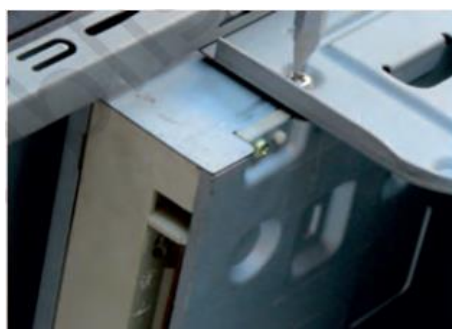
Fig. 4.26: Tighten screws of optical drive
