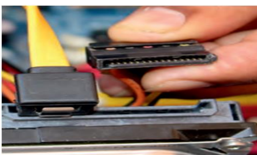
Fig. 3.20: Plug-in 15-pin connector to HDD
