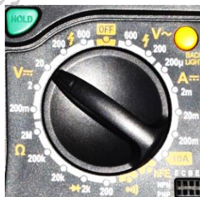
Fig. 4.26 (a) Turning the knob to measure the DC voltage
