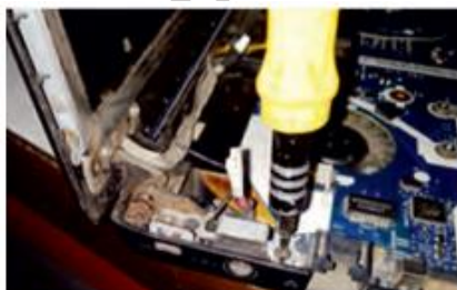
Fig. 3.72: DC power jack mounted under display hinge
