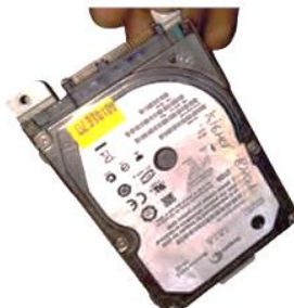
Fig. 4.22: Remove old hard drive assembly
