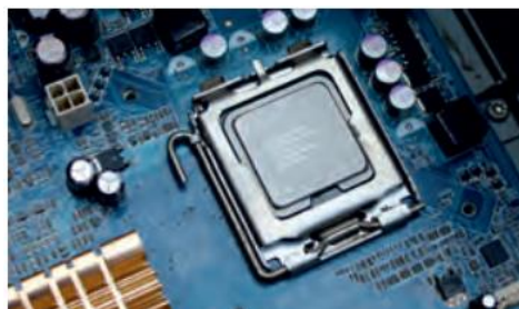
Fig. 3.5: Installing CPU on the motherboard
