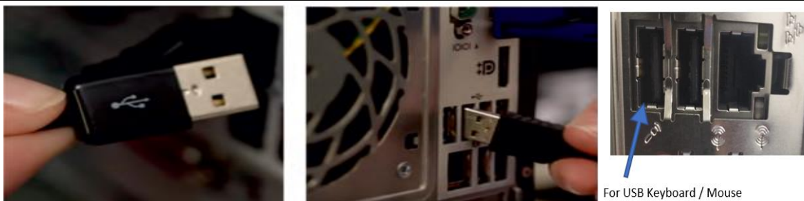
Fig. 3.26: Connecting keyboards in USB port
