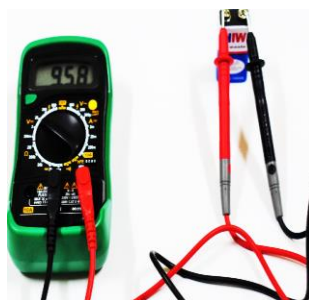
Fig. 4.28 Measuring DC voltage using multimeter
