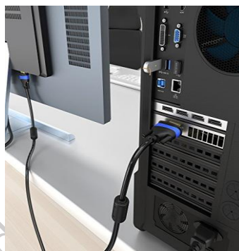
Fig. 3.24: Connecting VGA or monitor cable to the port on back panel of computer
