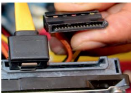
Fig. 3.41: Unplug 15-pin connector from HDD
