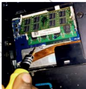
Fig. 3.66: Remove RAM memory modules
