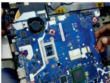
Fig. 3.74: Disconnect cable from motherboard and remove screws
