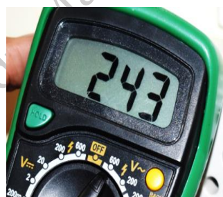
Fig. 4.29 Holding the value in the display using hold button
