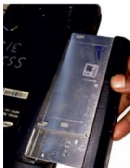
Fig. 3.68: Remove optical CD DVD drive connector board
