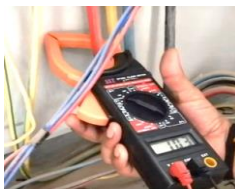
Fig. 4.20 Taking the reading on the clamp meter
