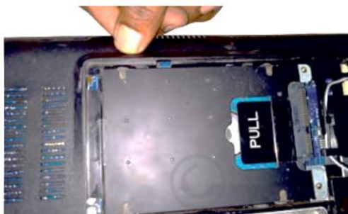
Fig. 4.21: Open connector and release hard drive cable
