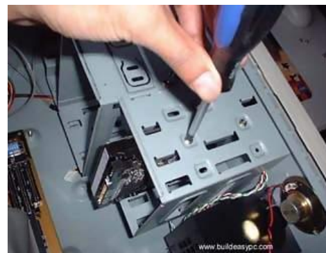
Fig. 4.14: Screwing the hard disk drive
